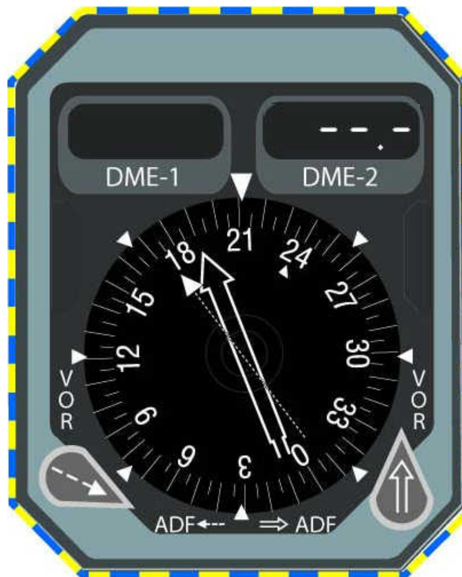
Figure 31 DME Fault and NCD Indication on DDRMI
